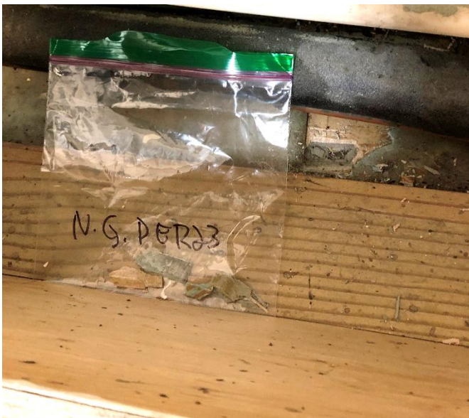
Asbestos Containing Gray VFT 12"x 12" with layer under with Mastic all under Ceramic Tile, Room 1-4
