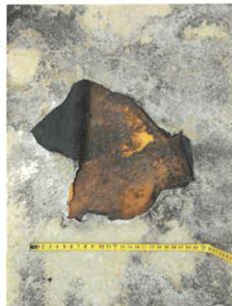
Roof, 9,600 SF of built-up membrane roof waterproofing treatment, 120 FT long x 80 FT wide, high winds, wind driven rain, and wind blown debris detached, bubbled, and peeled off the treatment, 0% work completed (photo 2 of 2)
